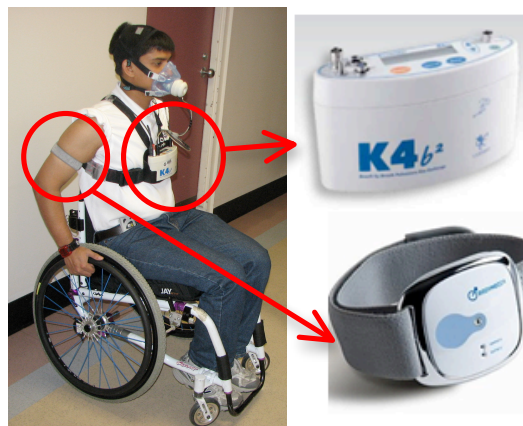
Figure 1: Each participant wore the metabolic cart K4b2 device (right top) at the chest area and a facial mask and the SenseWear armband (right bottom) on the dominant arm while performing each activity.
